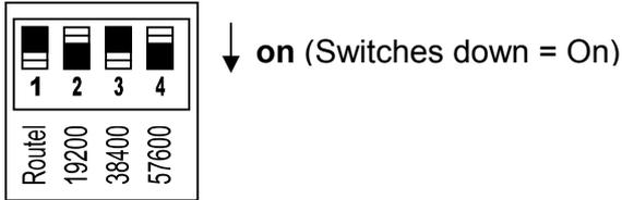
Setting switch 1 to 'on' (Switches down = On ) enables the Routel mode (dialling enabled).
